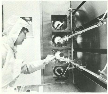
ELAINE HURLEY (2141) prepares a glass boat load of silicon wafers for high temperature diffusion inside a diffusion furnace, one of 17 in the lab. Temperatures range from 400° to 1200° C.
